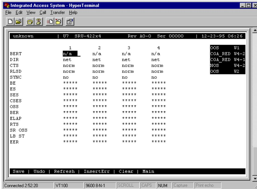
Figure 2-10. Typical SRU Card Test Screen
