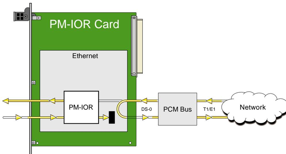
**Figure 6-4. Local DTE Loopback**
