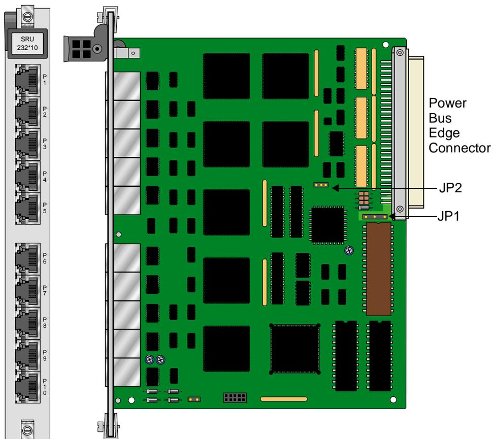
Figure 2-2. SRU 232\*10 C&D Bus Jumper Settings
