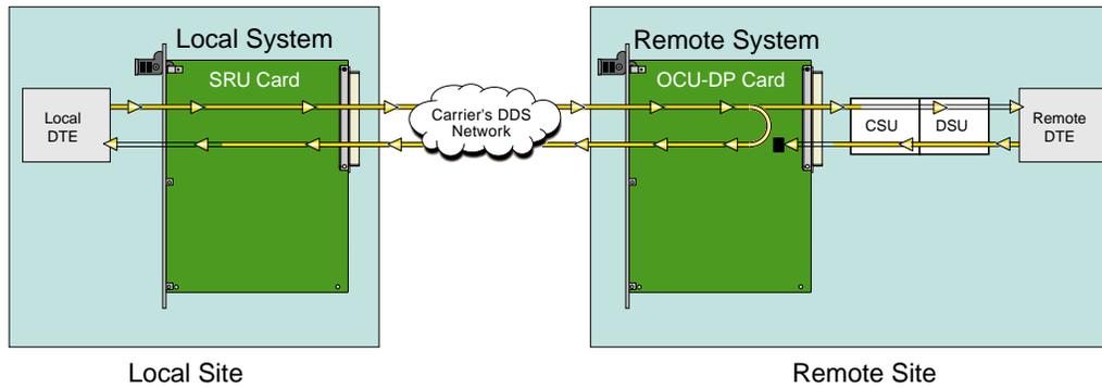
Figure 2-6. Inband Remote SRU Loopback
