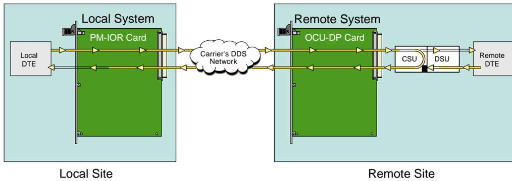
Figure 6-7. Remote CSU Loopback
