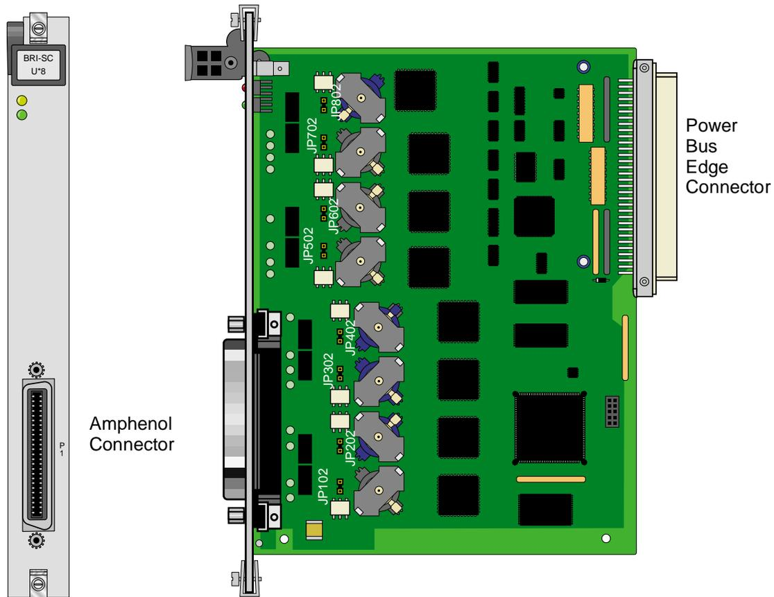
**Figure 5-3. BRI-SC U\*8 Card Sealing Current Jumpers (826170/71)**
