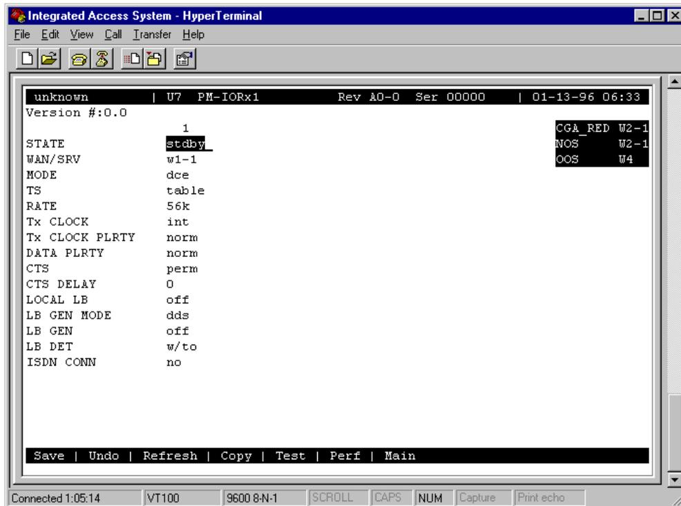
**Figure 6-2. Typical PM-IOR Card Main Screen**
