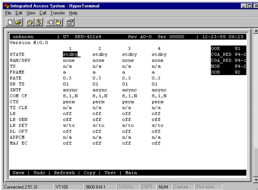
Figure 2-3. Typical SRU Card Main Screen
