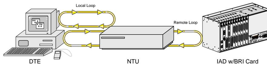
**Figure 5-14. Local and Remote Loopback Testing**
