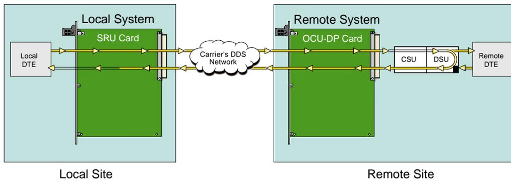
Figure 2-8. Inband Remote DSU Loopback
