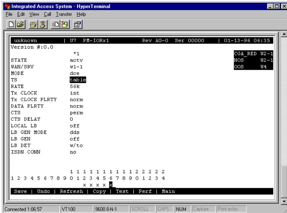
Figure 6-3. Typical PM-IOR Port time slot Assignment Screen
