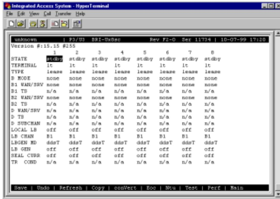
Figure 5-4. Typical BRI U\*8 and BRI-SC U\*8 Card Main Screen
