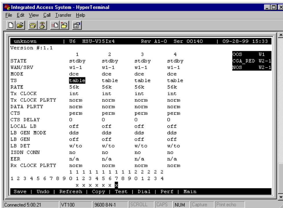
**Figure 1-9. Typical H5U Port Time Slot Assignment Screen**
