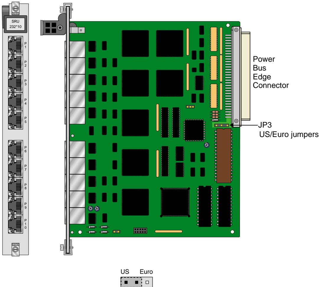
**Figure 2-1. SRU 232\*10 Jumper Settings**
