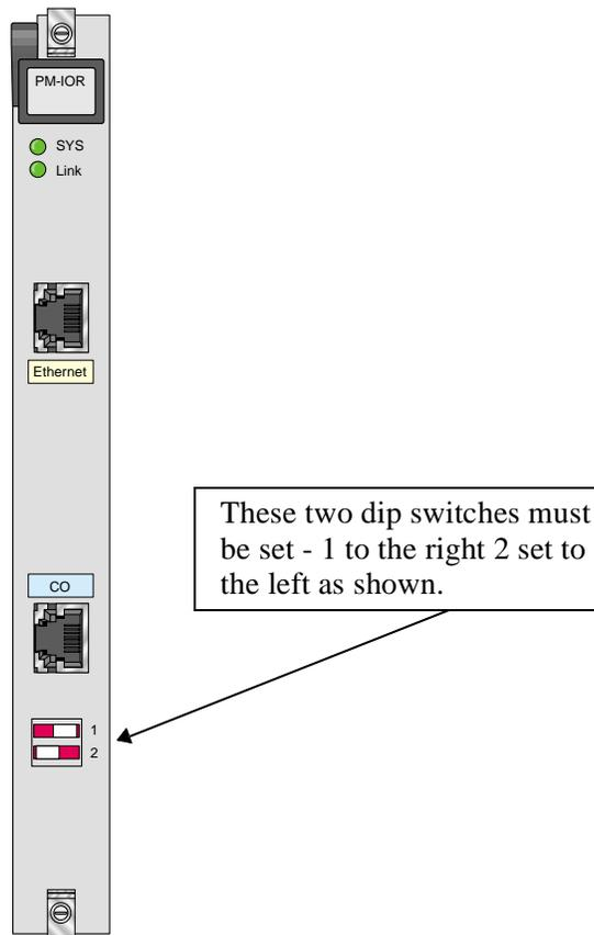
**Figure 6-1. PM-IOR Card Dip-switch settings (828060)**
