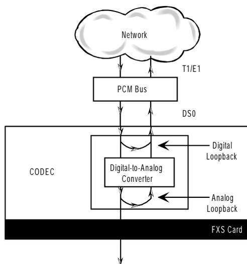
**Figure 2-4. FXS Card Loopbacks**
