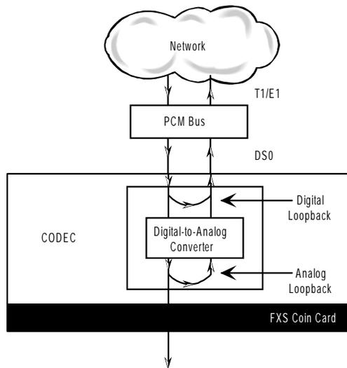
Figure 4-4. FXS Coin Card Loopbacks
