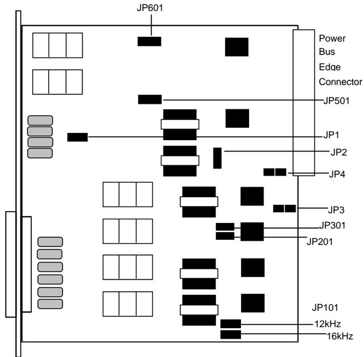
**Figure 4-1. Jumper Settings for FXS Coin Card**
