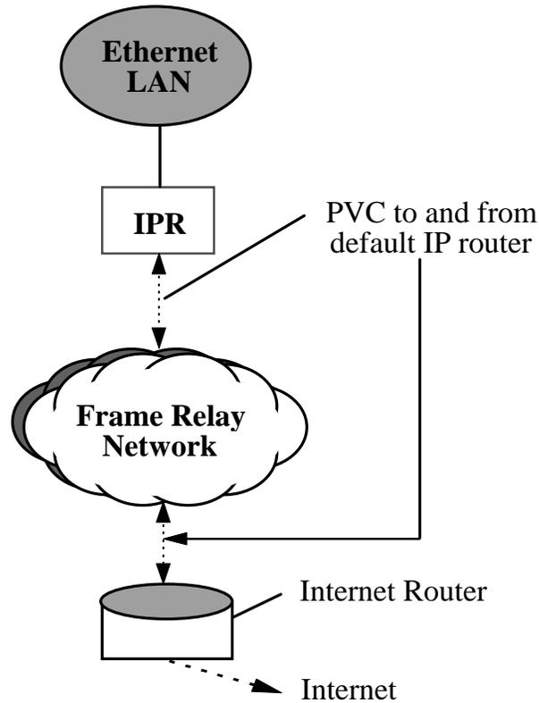
Figure 8-3. IPR Card Routed to the Internet through Frame Relay Network
