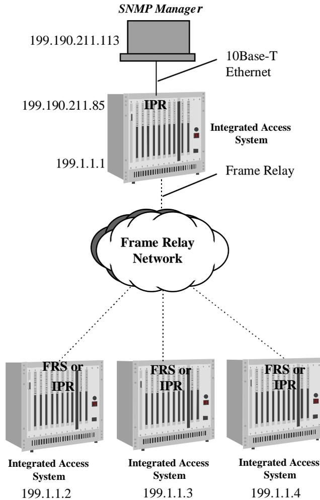
Figure 8-4. IPR Card Connected to IP Nodes on Ethernet to Frame Relay Network
