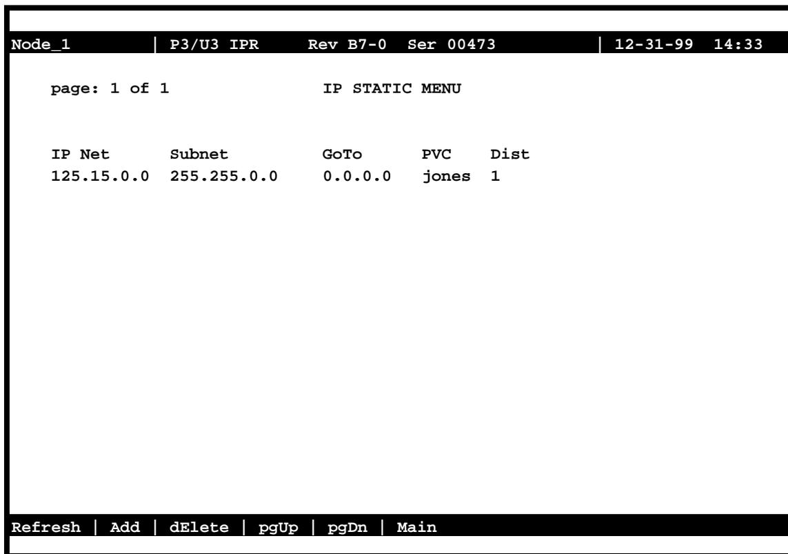
Figure 8-20. Typical IP Static Routes Configuration Menu Screen
