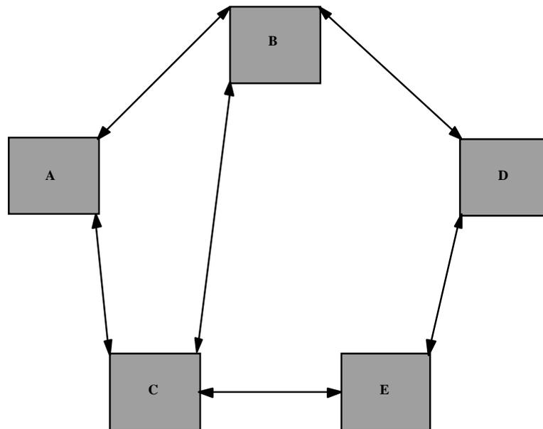
**Figure 8-7. Partially Meshed Frame Relay Network without Full Connectivity (Same IP Network)**
