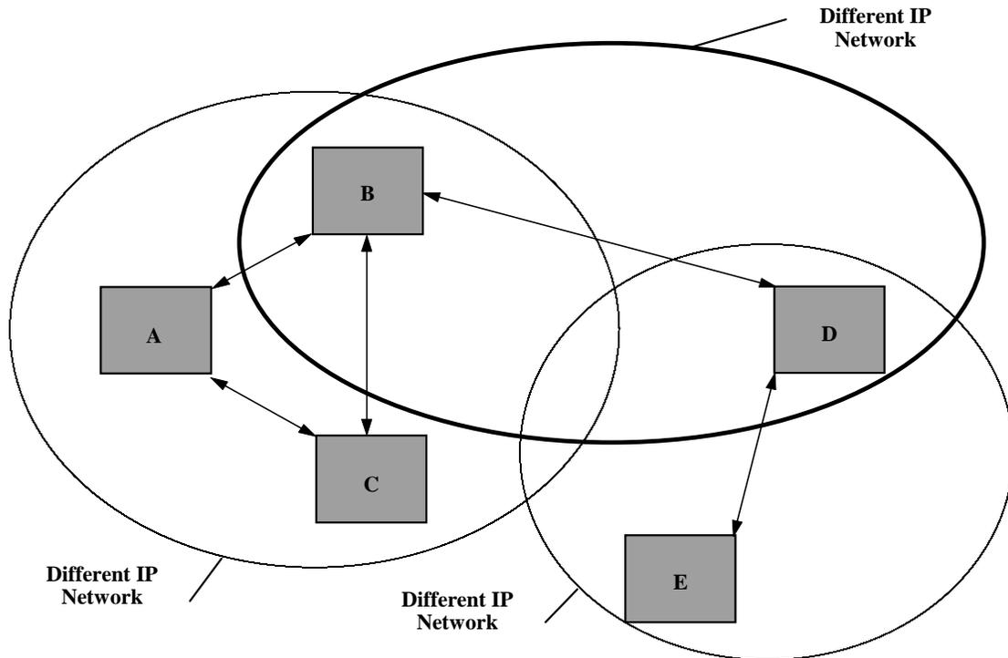
**Figure 8-8. Partially Meshed Frame Relay Network with Full Connectivity (Different IP Network)**
