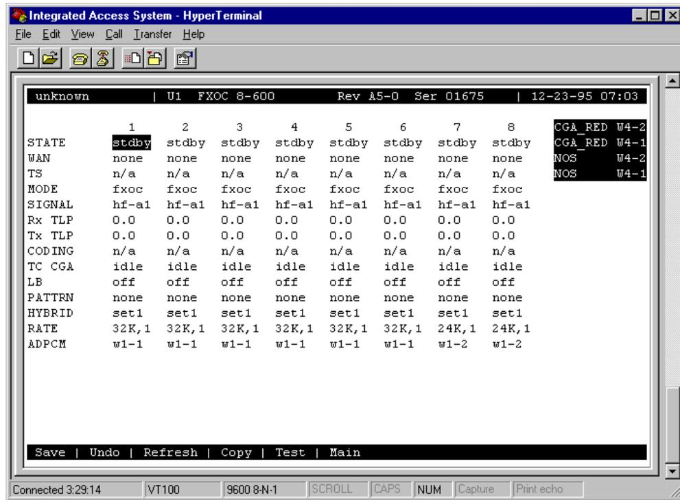
Figure 5-2. Typical FXO Coin Card Main Screen
