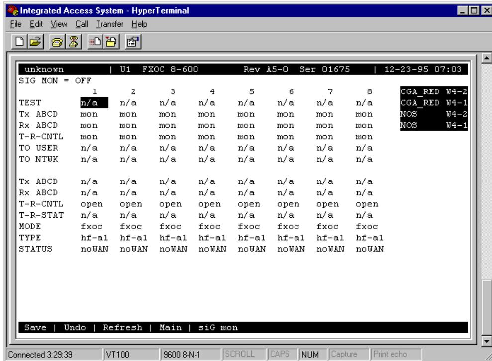
Figure 5-4. Typical FXO Coin Card Test Screen
