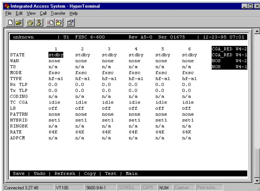
Figure 4-2. Typical FXS Coin Card Main Screen
