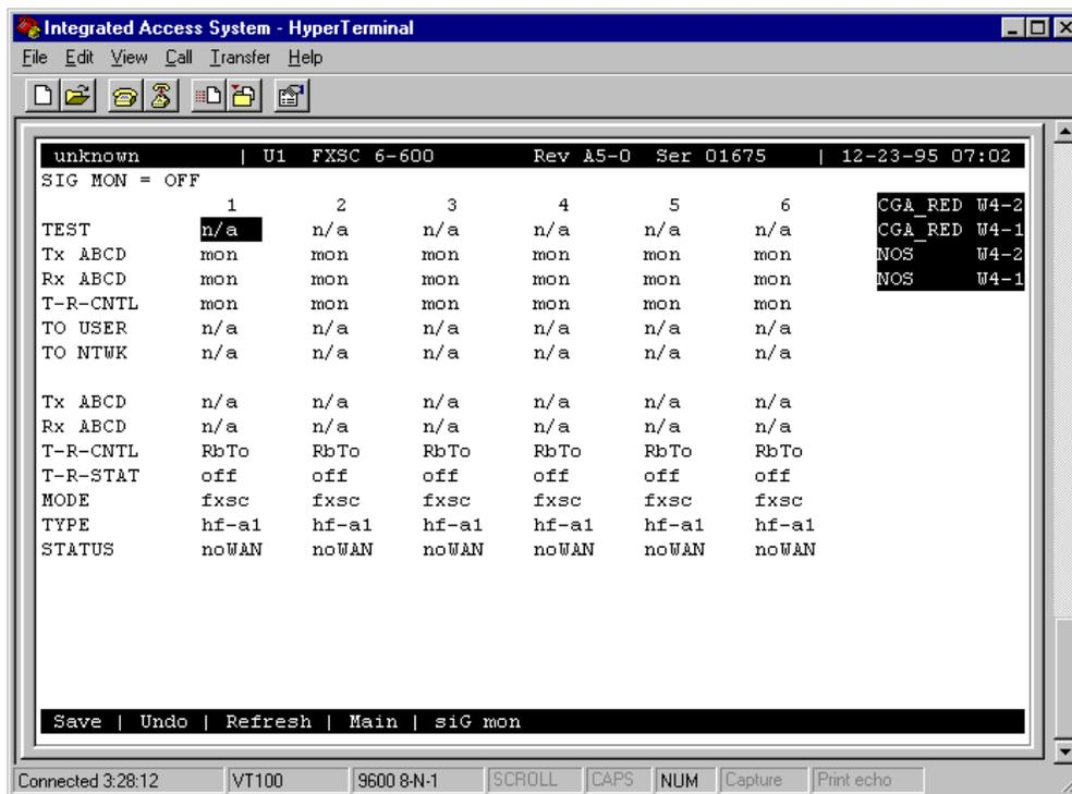
Figure 4-4. Typical FXS Coin Card Test Screen
