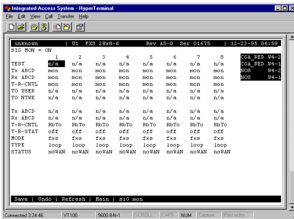
Figure 2-4. Typical FXS Card Test Screen
