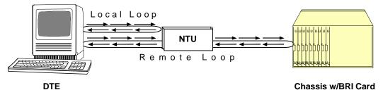
Figure 7-16. Local and Remote Loopback Testing
