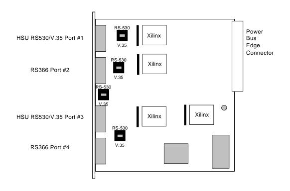
Figure 1-12. Four-Port HSU 530/35 Card Switches
