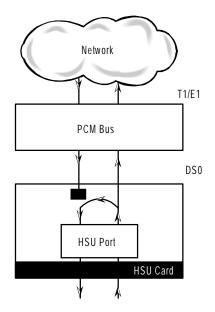
**Figure 1-19.Local DTE Loopback**
