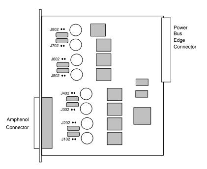
Figure 7-4. BRI-SC U\*8 Card Sealing Current Jumpers
