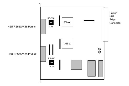
Figure 1-1. Two-Port HSU 530/35 Card Switches
