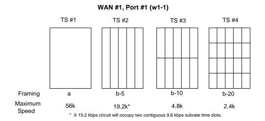
Figure 3-5. Data Frames, Rates, and Time Slot Assignments
