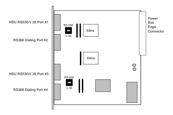
Figure 1-6. HSU-AD 530/35 Card Switches
